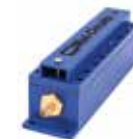
Case Style: ME1656 4.4 x 1.1 x 0.9" SMA-F connectors
