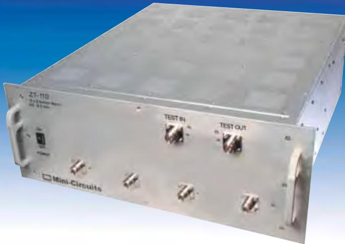
THE ZT-110 high performance switch matrix is designed to handle 40W of transmit (Tx) power from an RRH and simultaneously work with the receive (Rx) path of another channel. This configuration eliminates the need to turn off the high output power in the Tx path during channel swapping. A built-in isolator provides additional signal isolation between the Tx and Rx paths. Current configuration operates over 2000 – 3800 MHz. Other frequency bands are also available upon request.
