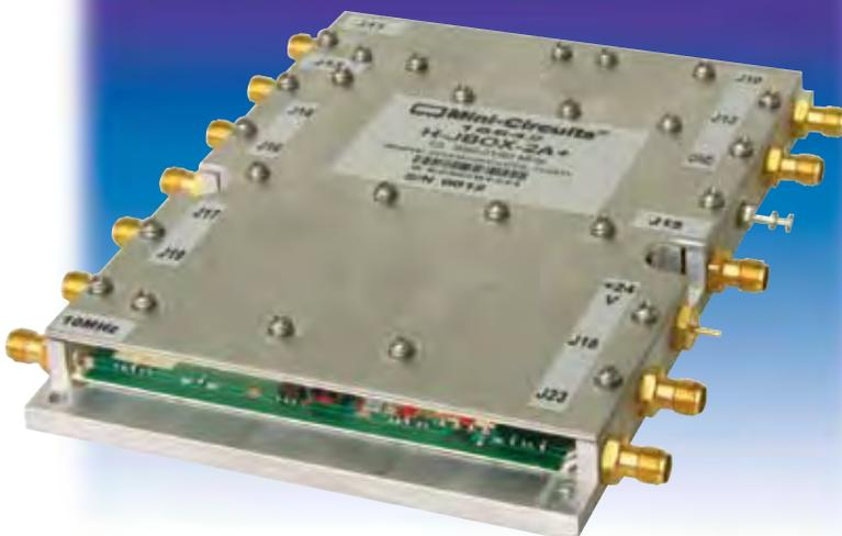
The Mini-Circuits J Box is an L band diplexer featuring two receive paths and two transmit paths. The receive paths have approximately 30 dB of forward gain, and both are designed with a 2 way power splitter on their inputs to drive multiple modems.
